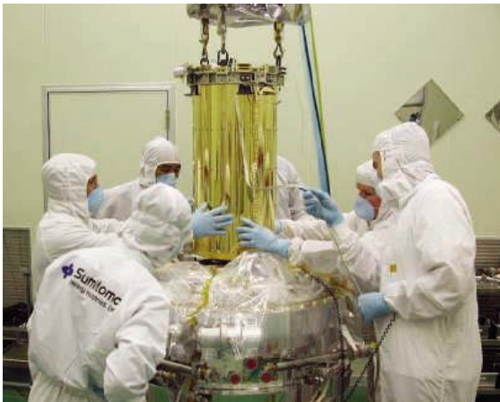
Dewar die. The inability to maintain a vacuum doomed the lead instrument on Suzaku.
